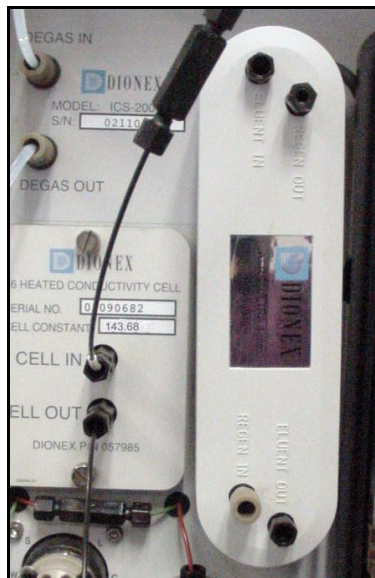
Figure 20. Suppressor Installed (SRS Shown)
