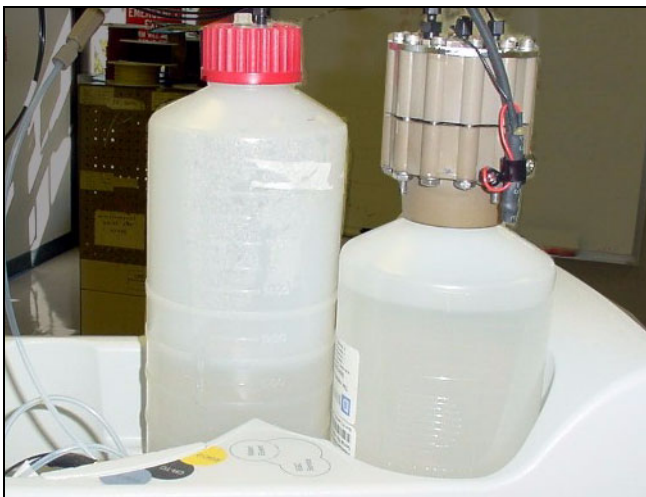
Figure 35. EGC in Service Position
