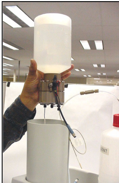
Figure 39. Installing the EGC in the Holder
