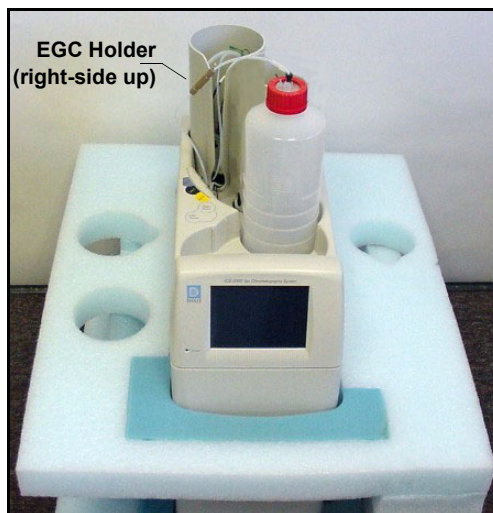
Figure 2. ICS-2000 After Installing Eluent Bottle and EGC Holders
